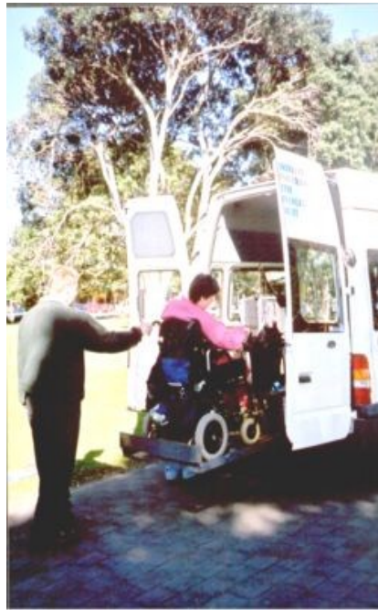
Trish is lifted into the van using the hydraulic hoist.
